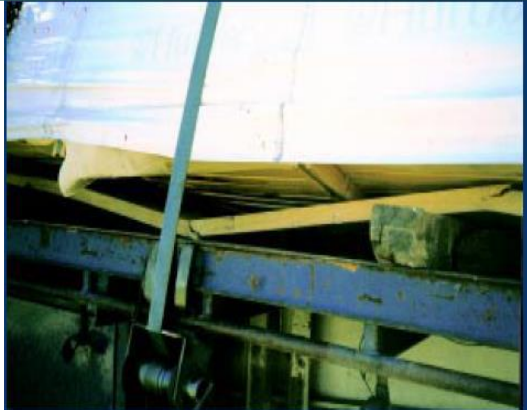
The base of the load broke from the strapping tie-down force. The strap should have been positioned above the dunnage supporting the load. (Photo courtesy Queensland Transport).
