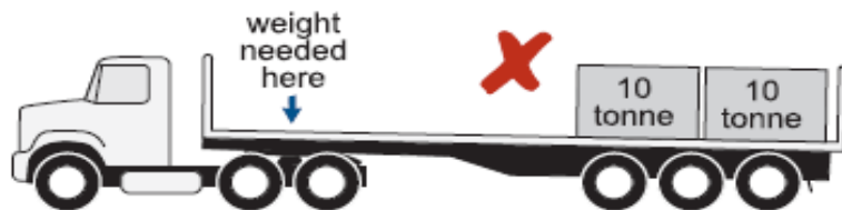
Fig. B.10 INSUFFICIENT WEIGHT ON DRIVE AXLES
